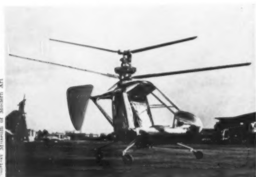
A mass-produced, low-cost helicopter has been an elusive goal for years. This prototype, with cab of molded plywood, was designed in 1945 by Alvin Lustig for Roteron.
