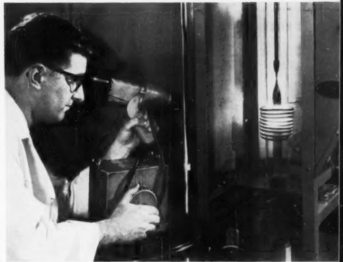
To make silicon rectifiers, material must be ultra-pure so that amounts of impurity that must be added for rectifying action can be controlled. At Raytheon silicon crystals are “grown” by immersing a silicon-tipped rod and slowly pulling it out.
