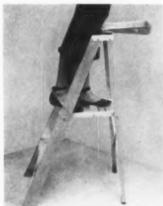
↑ Stepladder with stability, made by Howard B. Rich, Inc., has extra wide center step, knee-bar brace to lean against. Made of aluminum, it folds flat, will take roll-on paint trays. In 4, 5, 6-foot heights.
