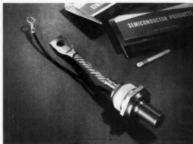
GE's silicon controlled rectifier not only changes ac to dc, but controls amount of current fed into circuit. This new 50 amp unit is 2 inches high, weighs three ounces.
