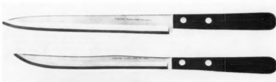
† Robeson "Flame Edge" cutlery has a thin layer of tungsten carbide fused to one side of steel blade. As steel wears, more tungsten carbide is exposed, so that knife sharpens in use. Staff design, Jerome Moberg.
