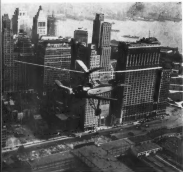
Early autogiro, designed by Cierva and manufactured in U. S. by Pitcairn. Some later models eliminated wings.
