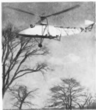
Igor Sikorsky in VS 300, first successful helicopter in U. S. Machine was tethered for first year while inventor learned principles of control. Rope was cut in 1940.
