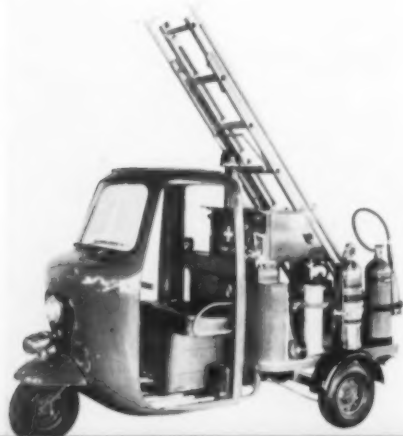
Lambretta Firefly can be used in factories, institutions, and/or civil defense. It includes ladder and extinguisher.
