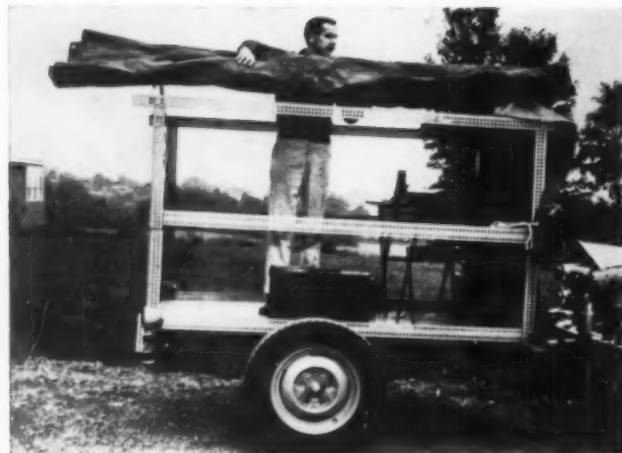
Varying the arrangement and amount of metal lumber, a flatbed trailer develops into a boat trailer able to support a 14-foot boat. Another tier of lumber converts this into a one-man office (left) and finally to a double-decked camp trailer sleeping four.
