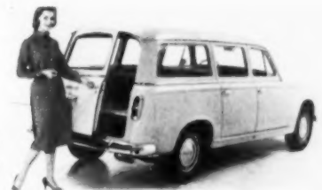
Peugeot 403 is 15'1" in overall length and has 114" wheelbase. Its price is $2490.
