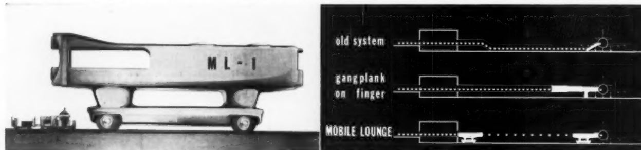
Design for mobile departure lounge (below) cuts passenger walking distance to a minimum as contrasted with older systems (below).
