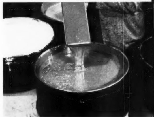
The coating is applied to the new → mill product in the form of liquid vinyl plastisols inspected here before use on coated sheet production.
