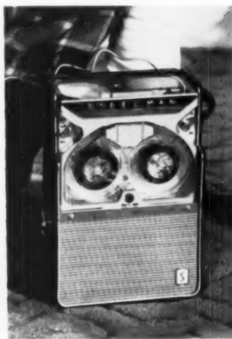
← Steelman Transitaape, two-speed tape recorder designed by Monte Levin, uses batteries, transistors, to achieve portability. Weight: 6½ pounds.
