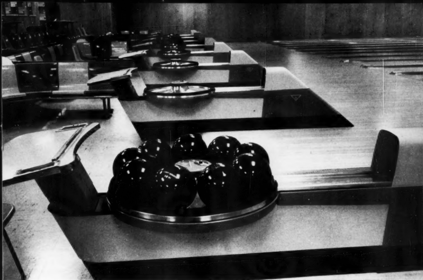
"Magic Circle" ball-rest (above) turns around stationary hub containing hand-dryer. Trough is stainless steel with black vinyl bumper; underside is heavily coated with sound-deadening compound.
