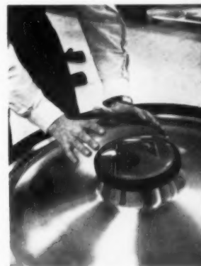
Hand dryer in center of turntable has push-button control, red "on" light; it also contains new triangular insignia in See-Deep plastic.
