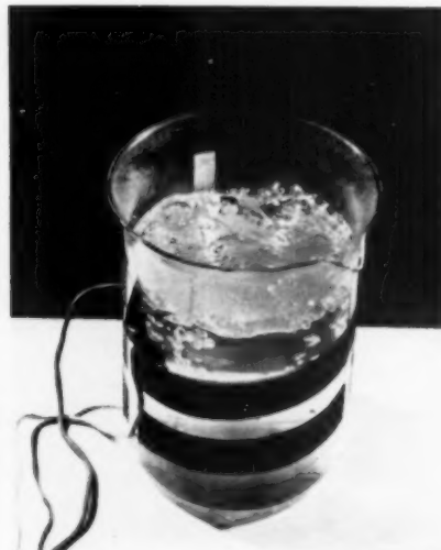
Top: Woven graphite fibers shown above in several weaves; immediately below, fibers used as lamp filament; right, as heating element.
