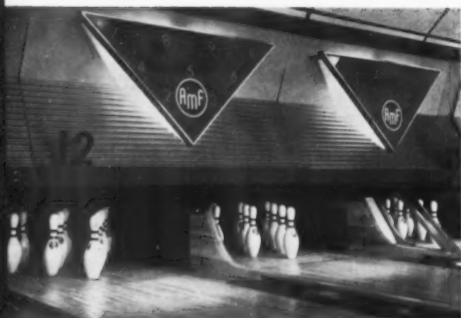
New Pindicator (above) is three-dimensional in contrast to linear quality of old Pindicator (right). Triangular shields float in front of angled back panels, and are set off by diffused side lighting. Top of back panel is mat gray, bottom is gilded, corrugated steel.
