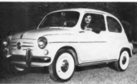
Fiat 600 sedan has 21.5 hp and a wheelbase of 78.75". It gets over 30 miles per gallon of gasoline. Price: $1398.
