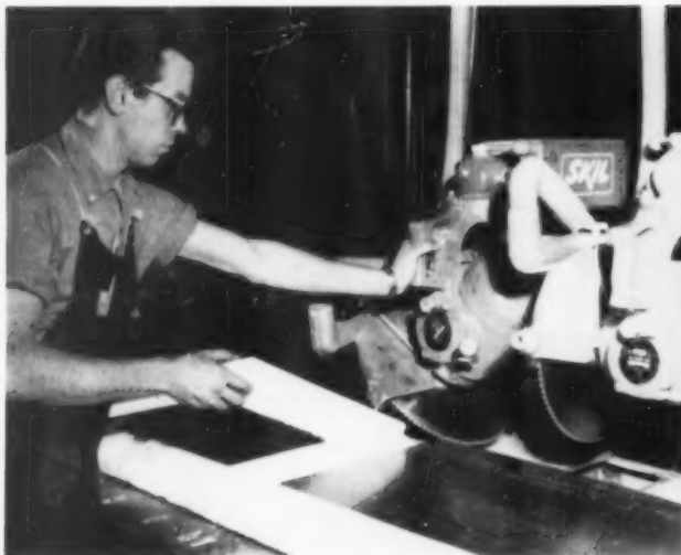
1. Panel being notched and mitered with high speed saw.
