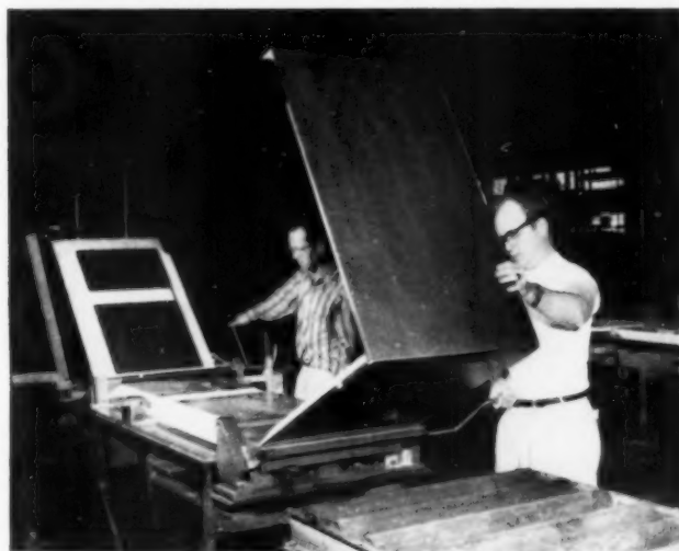
3. Assembling top, bottom and two sides of refrigerator.
