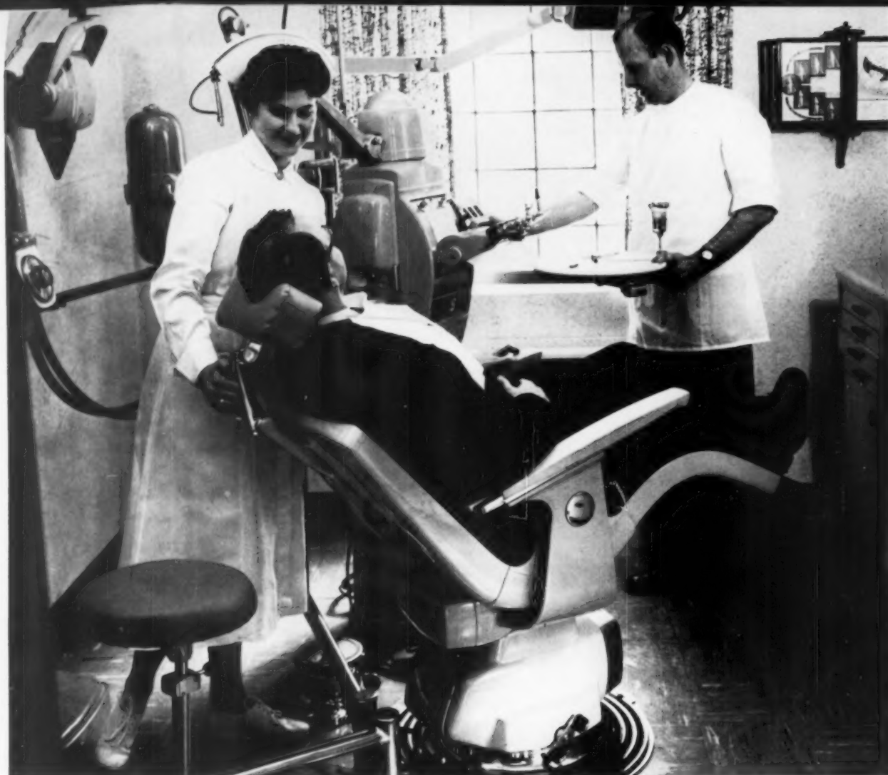
Euphorian dental chair puts patient in reclining position with his head low enough to allow dentist to operate sitting down.
