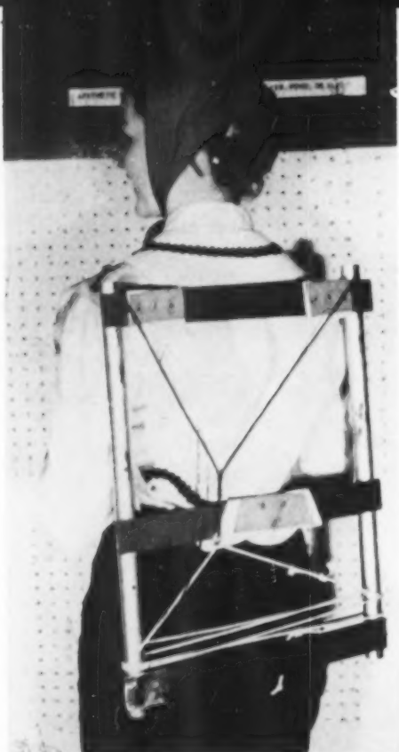
Harris Dunlap's knapsack frame, produced as part of the camping project, is constructed of aluminum tubing and is easily removable.
