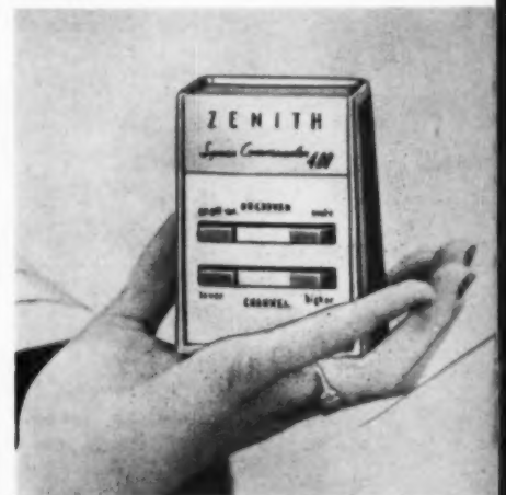
▼ Zenith Space Commander 400 tv remote control system is operated by ultrasonic impulses. System formed part of U.S. exhibit in Moscow.
