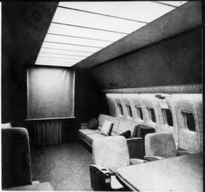
Inside "flying office" of Boeing MATS staff transport, Colovin laminate forms window panels, cove-light covers, curved overhead areas.
