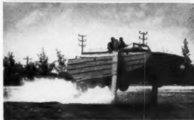
Hydrofoils exert lift, like wings.
