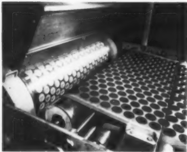
At Nabisco's new plant in Fair Lawn, N. J. all mixing operations are directed from this master console pre-set to deliver the required ingredients for numerous recipes. Nearly half a million cookies an hour are shaped by machine (left) before moving belt takes them into oven.
