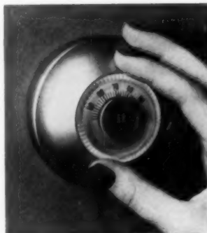
Simplest and most popular of temperature controls, the room thermostat, is now being extended to include air-conditioning control. The desired temperature is pre-set; any deviation is sensed by thermostat, which then puts the control cycle in motion. This round thermostat (Minneapolis-Honeywell, designed by Henry Dreyfuss) controls heat only; push-button unit (White-Rogers Company) looks after air-conditioning as well as heat.
