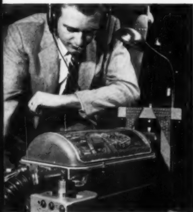
Missiles, inertial guidance systems, space platforms could not be planned were it not for gyroscopes and other sensing elements. This reference unit, or "inertial stable table" helps guide the USAF's supersonic B-58 Hustler. (Reference unit by Sperry Gyroscope Company.)
