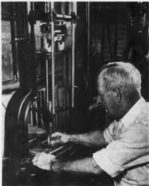
Benton Matrix Engraving Machine automatically contracts the width of larger letters and expands the width of smaller ones in relation to their heights to correct optical problems. Example: directly below, an 8 pt. Craw Modern Bold H enlarged photographically and, below that, a 72-point one cut on the machine.
