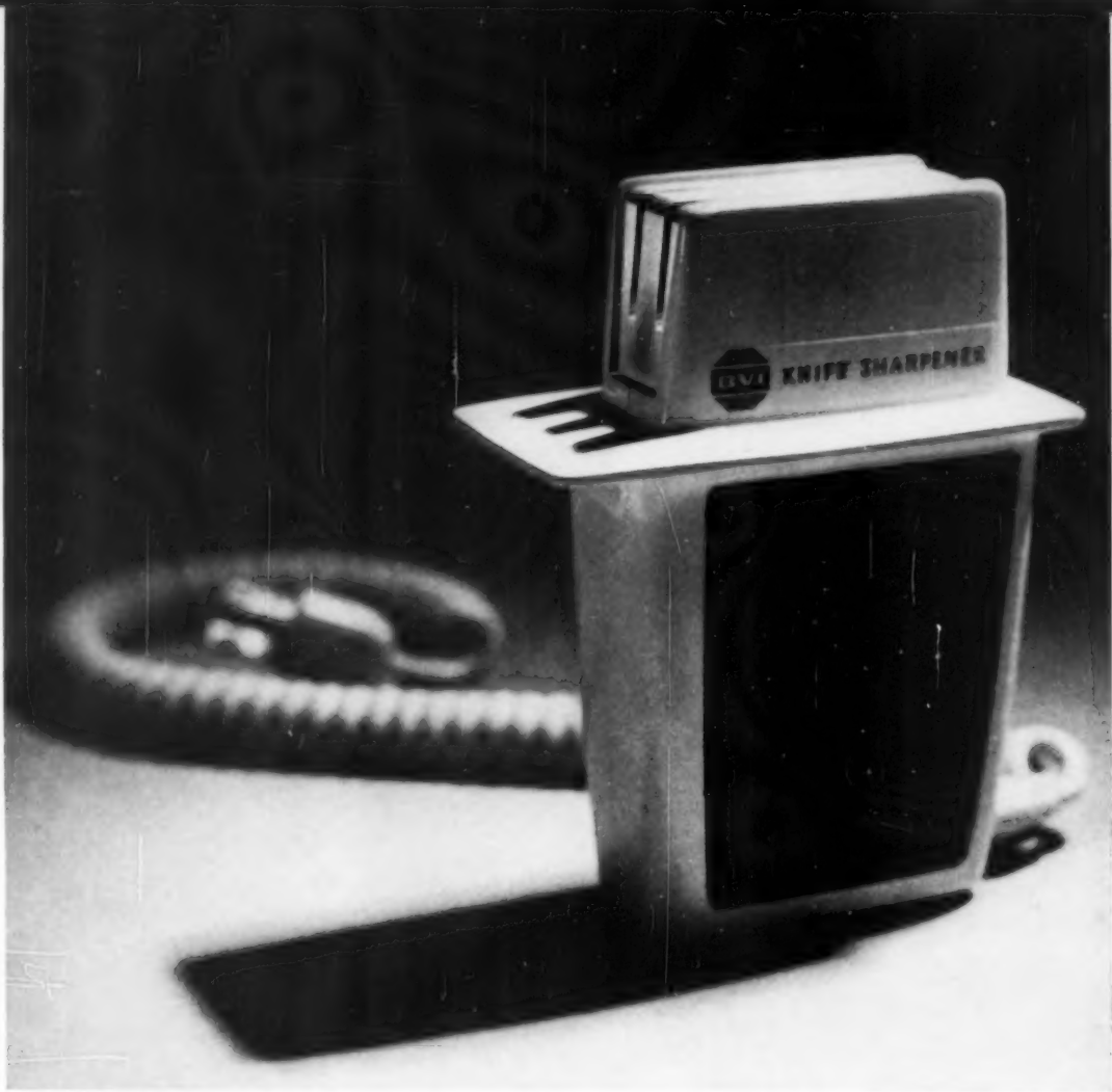
17 Electric knife sharpener Burgess Vibrocrafters, Inc., Grayslake, Ill. Dave Chapman, Inc. (Douglas Anderson), designers Conical carborundum stone operated by vibrating motor; contour design for convenient hand grip; extended lip for safety. Two-piece melamine housing; beige and brown; chrome-finished blade.
