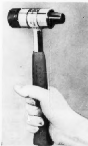
280 Hammer Olin Mathieson Chemical Corp., New York Hammer head suspended by elastic shocks within head housing; shock absorbent; non- slip, non-twist, neoprene covered metal handle.
