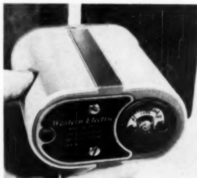
178 Portable frequency standard Bell Telephone Laboratories, Inc., New York For checking and readjusting a radio relay system oscillator; ten times more accurate than unit to be tested.
