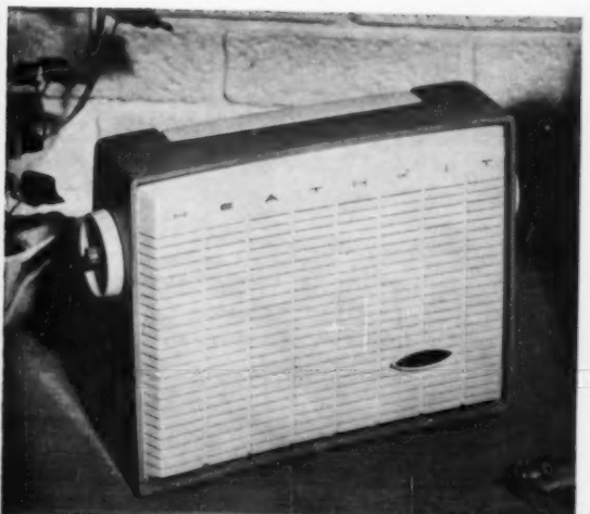
65 Transistor radio Sears Co., Benton Harbor, Mich. Hart Starr, staff designer Separate grille mounted to chassis allows for color and design changes. A-transistor circuit.
