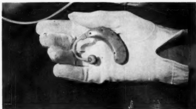
111 hearing aid Zenith Radio Corp., Chicago Miniaturization of component parts results in smaller "behind-the-ear" hearing aid. two mike openings for use at either ear.
