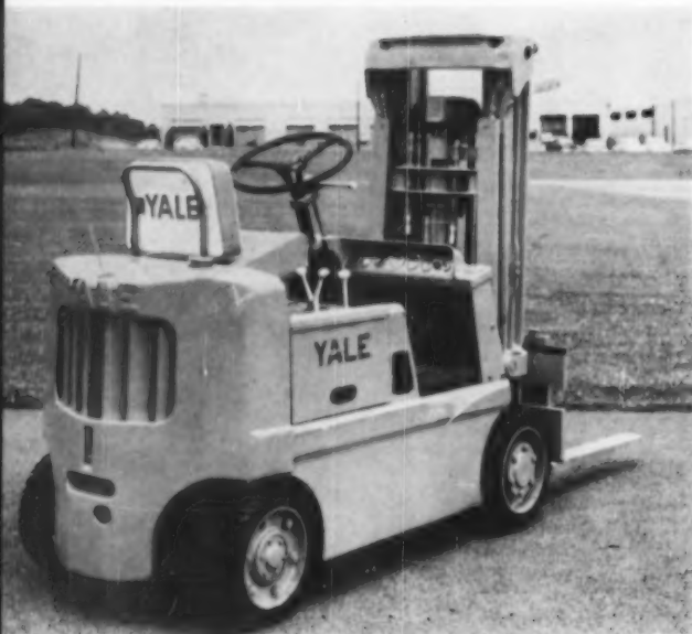
251 Gas truck Yale & Towne Mfg. Co., New York Adjustable, foam rubber seat; suspended dual brake pedals; separable instrument panel unit.
