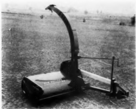
256 Crop-chopper New Holland Machine Co., New Holland, Pa. C. J. Kermes, product stylist Sheet metal dividers separate standing crop from wheat being chaffed.
