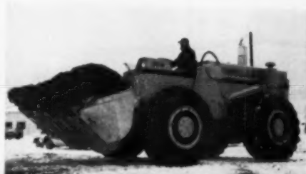
264 Trojan tractor shovel Yale & Towne Mfg. Co., New York Charles J. Jacobus, Chief Engineer One piece side plate to avoid weld undercuts in stress areas; front bumper integral part of frame.
