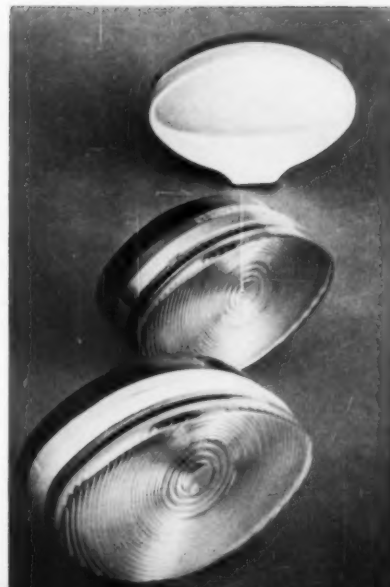
137 Rear view mirror Jervis Corp., Detroit Switch adjusts mirror up, down, or sideways. Stainless steel cables by Allegheny Ludlum.
