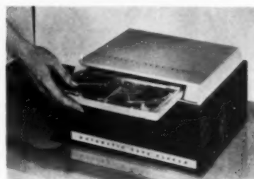
85 Continuous-play tape magazine Conley Electronics Corporation, Skokie, Ill. Magazine slips into player slot to provide automatic continuous performance. Tape in cartridge forms continuous loop, unwinds from single spool at center, automatically rewinds on outside of spool.
