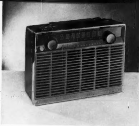
59 Transistor radio General Electric Co., Bridgeport 1957 design; Eric C. Rosenfeld, designer; W. S. Donnelly, assistant designer; D. L. Mulford, Manager, Industrial Design Operation Wide-area front supports entire chassis assembly. Circular case with leather handles.
