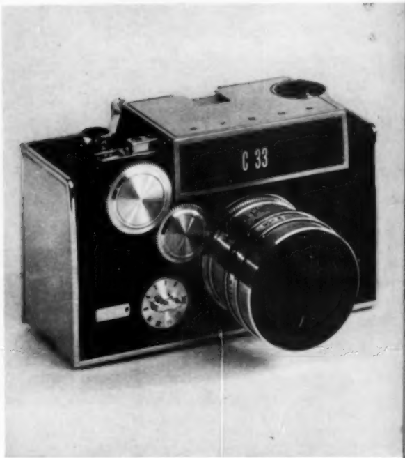
118 C-33 camera Argus Company, Ann Arbor, Mich. Harley Earl Associates (Ray Grosse), de- signers Interchangeable lenses coupled with single- window range-viewfinder. Zinc and alu- minum body.
