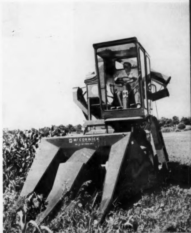
257 Harvester-thresher cab International Harvester Co., Chicago Tinted glass resists sun glare and dust accumulation. Automatic wiper and washer keep windshield clean.
