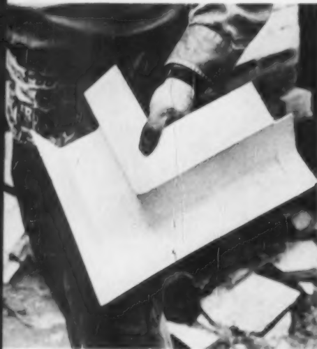
290 Gutter and downspout system. Owens-Corning Fiberglas Corp., Toledo Strong, lightweight "Fiberglas Perma- drain" roof drainage system will not rot, dent, rust, corrode, or split-freeze; can be nailed like wood; needs no painting. Made of Fiberglas-reinforced plastic. Shown, left to right: corner, cross-section, installation.
