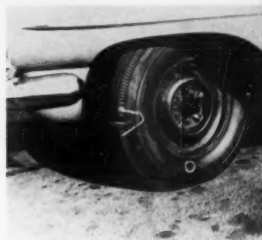
248 Solid tire Dayton Rubber Company, Dayton, Ohio Experimental prototype of plastic-foam-filled automobile tire that is blow-out-proof, airless, easy-riding.
