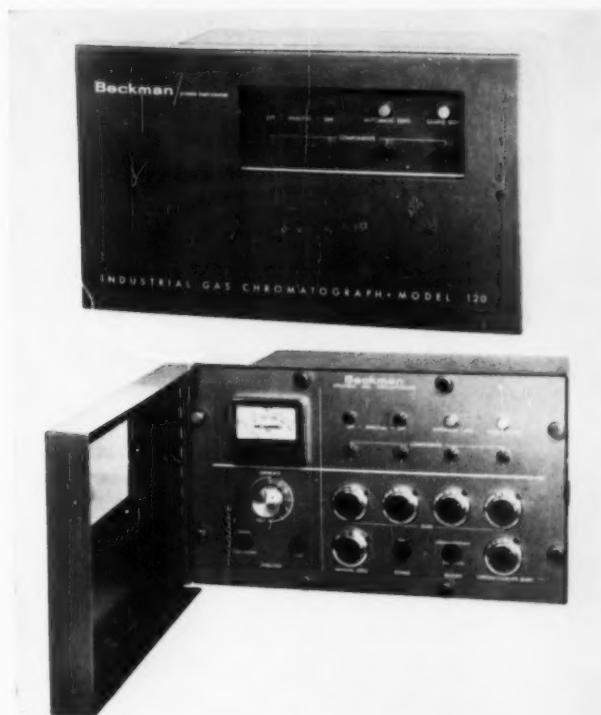
Door prevents accidental re-setting of controls once instrument is "on-stream," allows operator to view lights through window.
