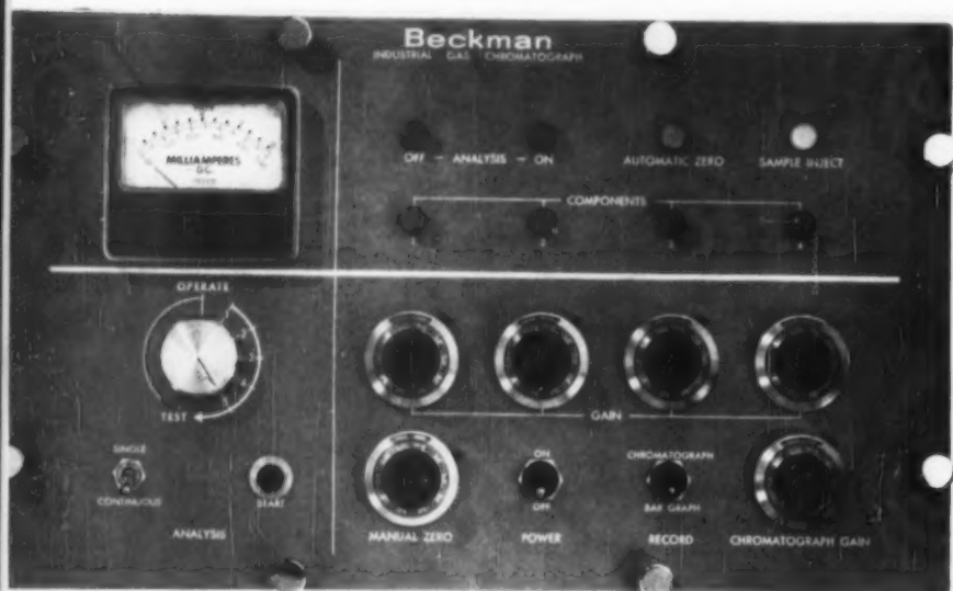
Controller redesigned. Four quadrants logically group visual readings (north), manual controls (south), programming/testing (west), and process checking (east).
