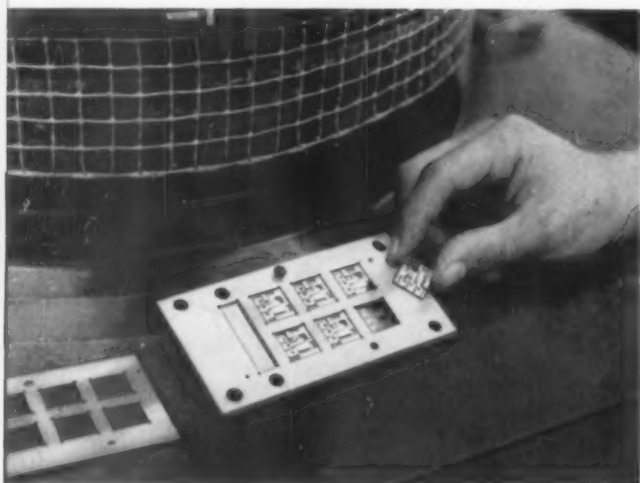
New micro-circuits, way ahead in miniaturization, consist of film of condensed metal vapors deposited on each side of glass substrate. At International Resistance Company, Philadelphia.
