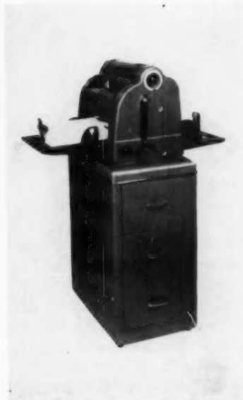
1946 Model 160 was first to use a semi-automatic inking device — a suction pump operated by a lever.
