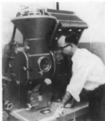
The crystalline structure of evaporated films changes with time and temperature. Process is observed through window of electron diffraction equipment at IRC.
