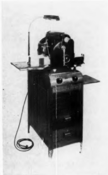
1933 First model designed by Loewy substituted automatic handle clutch for antiquated wheel.
