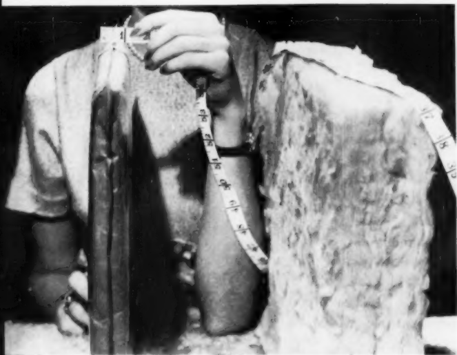
Hotpoint makes "Wonderwall," a plastic film and Kraft paper laminate, by inserting fiberglass batting into an envelope formed by the laminate. A charging chamber removes air from the envelope, forces a refrigerant in. Raymond C. Sandin, manager of design.
