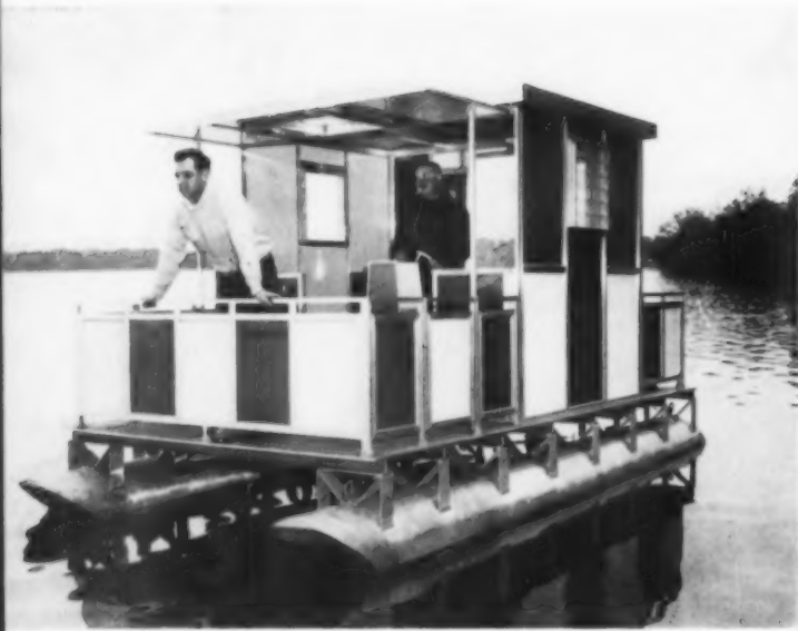
Construction is popular field for adhesives. Aluminum deck of houseboat (Imperial Mfg. Co.) is assembled with Williamson adhesives.
