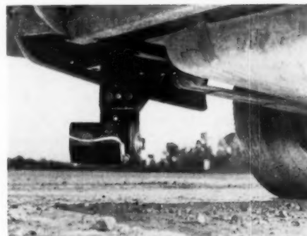
Surplus gun camera is ingeniously mounted under car to photograph effect of shock absorbers on wheel action, in picture produced by Video Films for Monroe Auto Equipment Co.
