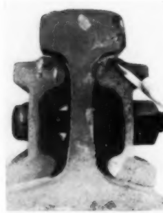
Void filling and joining adjacent parts is unique function of adhesives. In this rail joint adhesive fills void and joins bar to rail. Adhesive is by Armstrong Cork Company.
