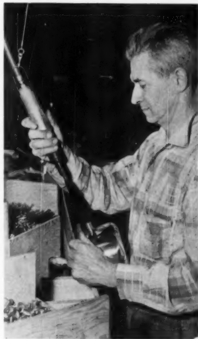
New handle not only looks simpler, but is simpler to assemble. It has fewer parts, can be mounted in fewer steps, requires no final brazing to mask joint.
