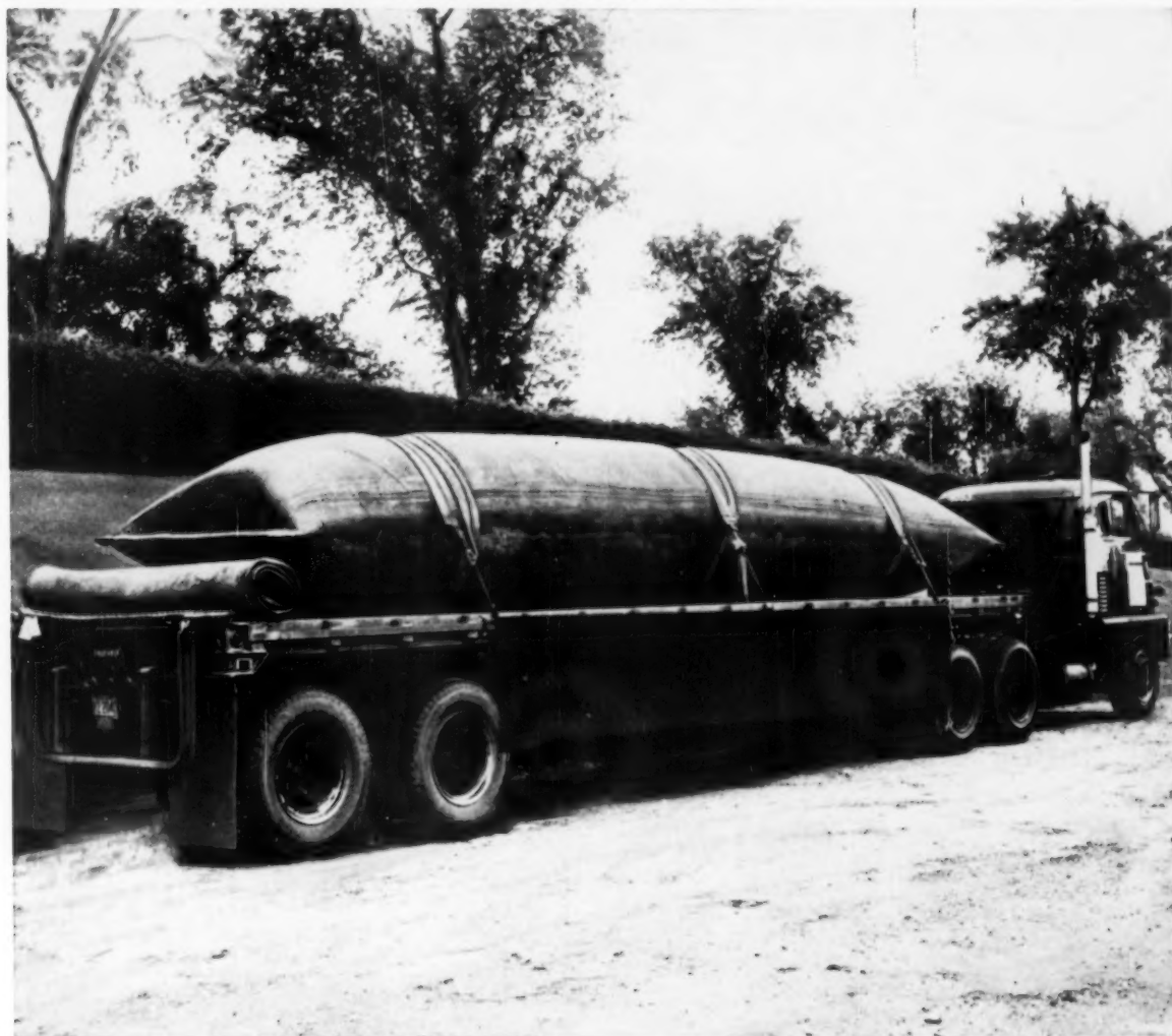
Flat-bed body which generally transports solid cargo is quickly converted to a liquid carrier... with a SEALDTANK*
