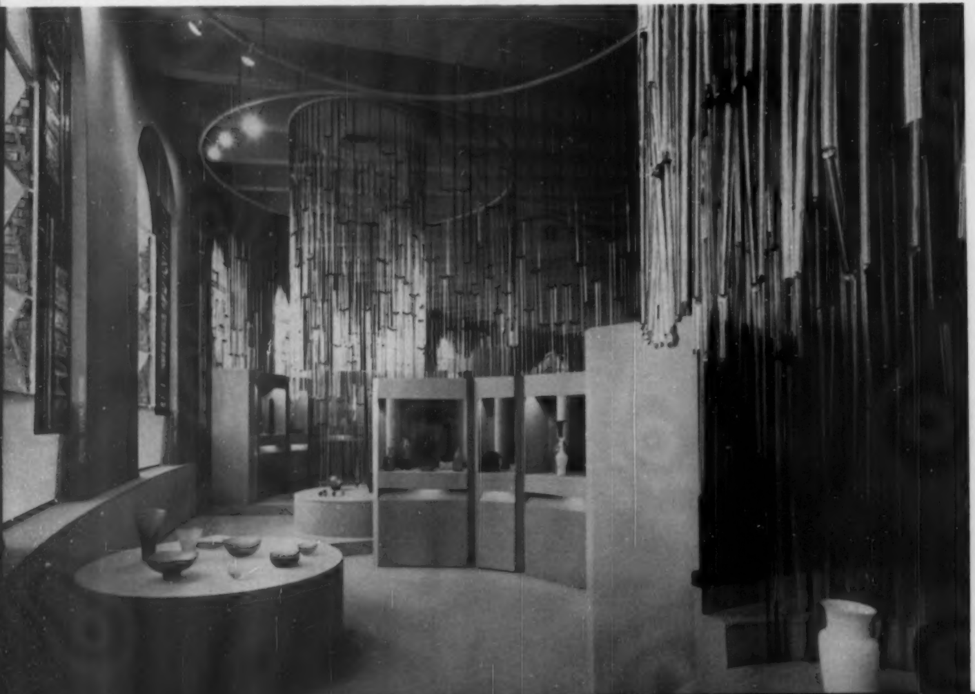
Backdrop for exhibit of Venini glass is curtain of glass tubes suspended from metal yokes. Designer: Roberto Menghi.
