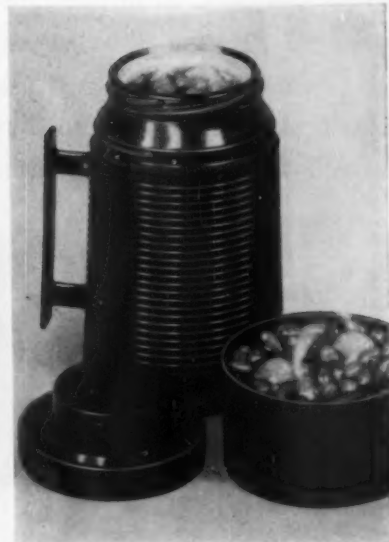
Aladdin Industries vacuum jug has handle and jacket molded in one piece from red polypropylene. Serving cup fits over screw-top lid. Ribbed exterior prevents slipping. Staff design.
