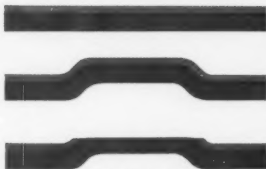
Duplex Butyrate sheet consists of a single thickness with thick and thin layers of Butyrate in two different colors.
