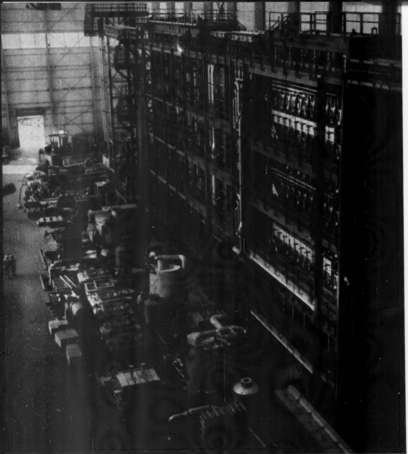
Continuous annealing line for tin plated steels. Courtesy U. S. Steel.
