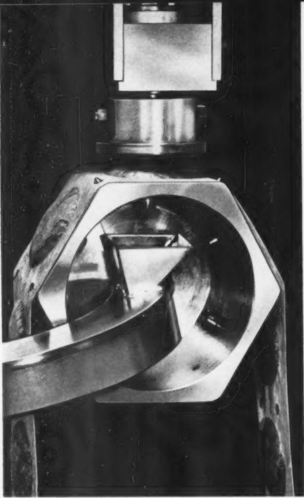
6—Rudd-Melikian's Brew-a-Cup coffee machine brews fresh coffee, one cup at a time, in six seconds. The coffee is pre-packaged in individual "pods," each carrying enough for a single cup, along a tasteless, odorless filter tape. At the drop of a dime, one pod of the tape is passed into a brewing chamber and hot water is passed through, perking the coffee into a cup waiting below. Liquid refrigerated cream and sugar are added automatically, if desired. The machine can also dispense hot chocolate, tea, and soup.
