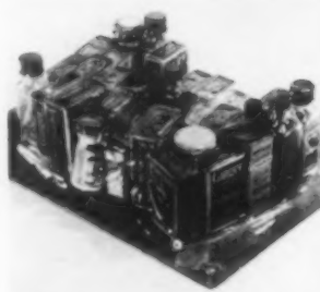
Some of the packaging films shrink to form skin-tight covers. Above, DuPont Mylar is used on smoked meats; below, polyethylene is used over a trayful of kitchen supplies to keep them from spilling in an innovation adopted by contract household moving companies.
