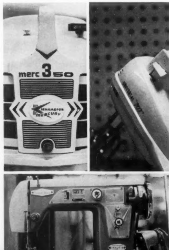
2. Meaningful and meaningless graphics as applied to an outboard motor (left), a hand mixer (right) or a sewing machine (below).
