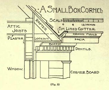
shown, forming a V shaped gutter lined with tin. A gutter of this shape allows the ice to collect without damage from lateral pressure. The mouldings in the angle between the soffit and the house wall are ornamental in their uses and are
