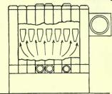
With The Burnham there is a flue between each section on both sides of the fire chamber. The flames come equally in contact with each section making every section equally efficient.
