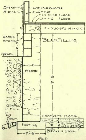
SECTION THROUGH BASEMENT WALL
