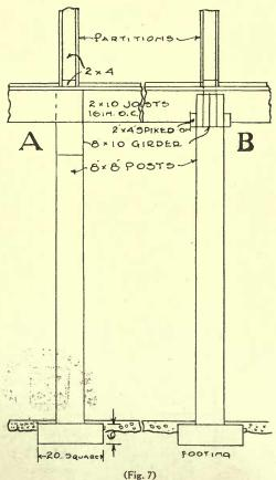
POSTS, GIRDERS AND FLOOR JOISTS
