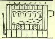
The arrows in this sketch show how boilers constructed with flue openings at back of boiler, draw the flames away from the front sections, impairing their efficiency.
