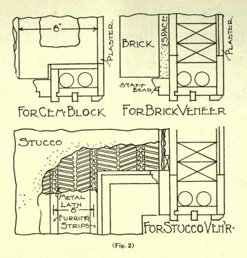
For brick veneer, staff beads take the place of the outside casings, as shown. It is made to receive the storm sash or screen 1½ inches thick.
