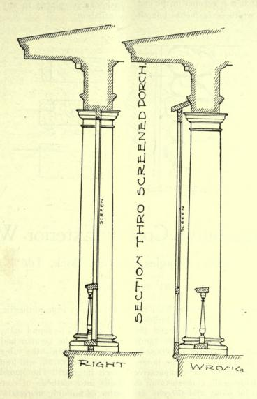
er screen is placed behind the balusters and below the bottom rail is a small filler of wood containing small holes at intervals to provide for drainage.
