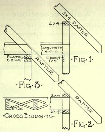
FRAMING OF RAFTERS, JOISTS AND PLATES
