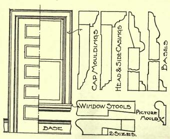
Fig. 2.—HALF ELEVATION OF DOOR AND WINDOW WITH DETAILS OF TRIM
