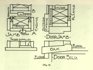
stud before plastering to make a good nailing place for the finish. In many cases grounds are omitted and the stop is not plowed in, but simply nailed flat to the jamb. The threshold is shown in position, but is being used less every day for inside doors.
