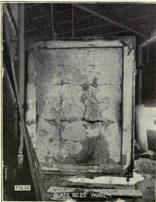
Metal Lath on Wood Stud after Water.
