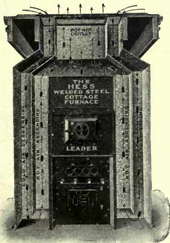
Hess Welded Steel Pipeless Furnace. One large register supplies heat and draws off cold air from the floor.
