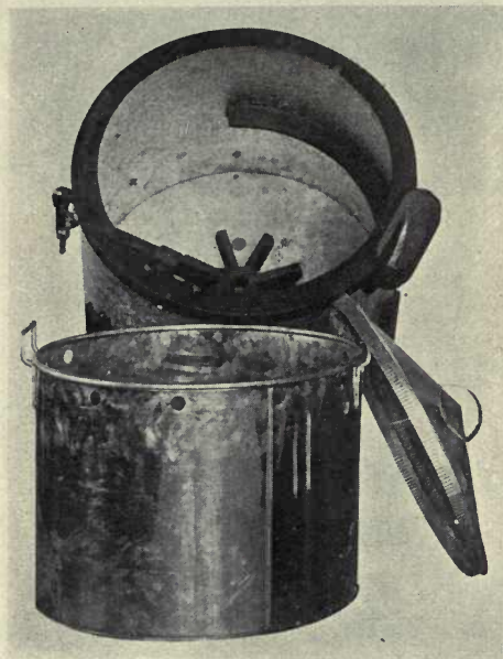
The outer shell enclosing burner and the inner vessel for the clothes.
