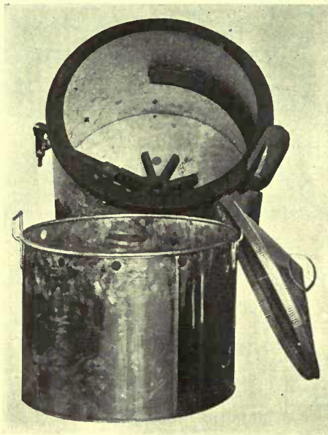
The vented outer shell enclosing burner and the inner vessel for the clothes.
