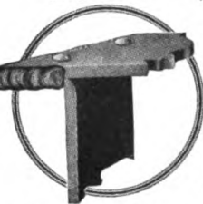
Section of welded flange type seam
