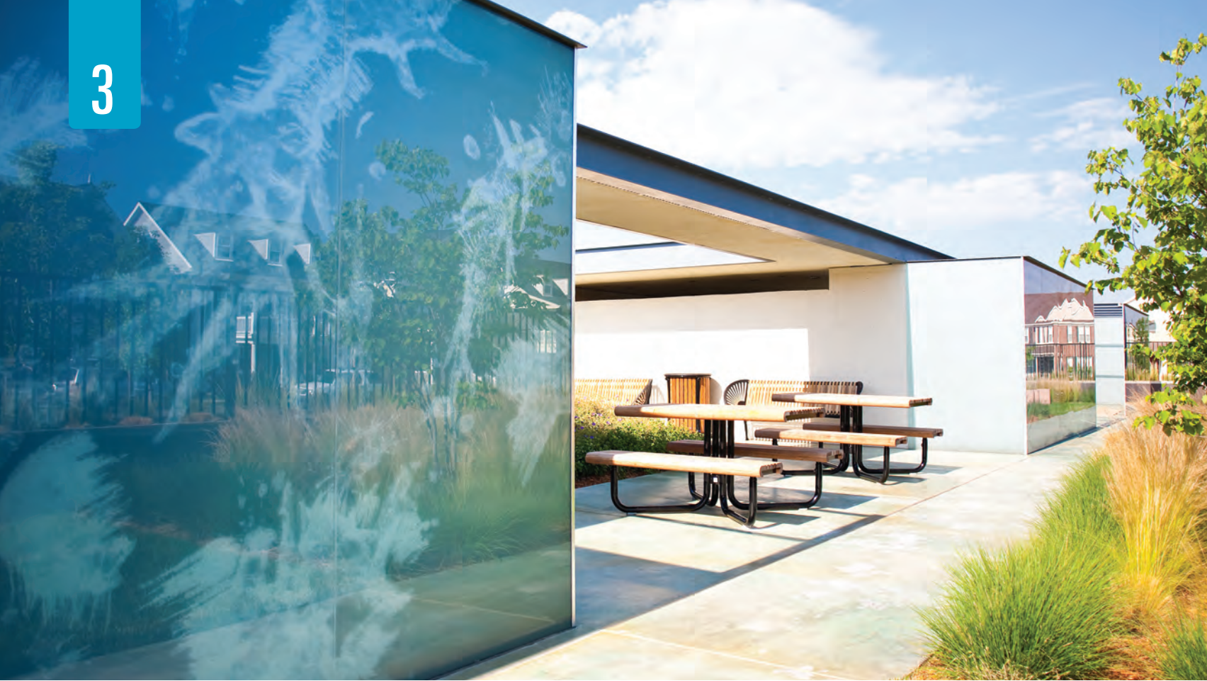
Pool House No. 3 was built using sustainable methods. The facility has no parking lot – only bike stations to encourage biking and walking. The roof collects rainwater and diverts it to the surrounding area. There is zero heating and cooling, and very little water-use. Three of the pool house’s pods are built using fly ash concrete, which reduces the amount of coal used to create concrete mixture.
