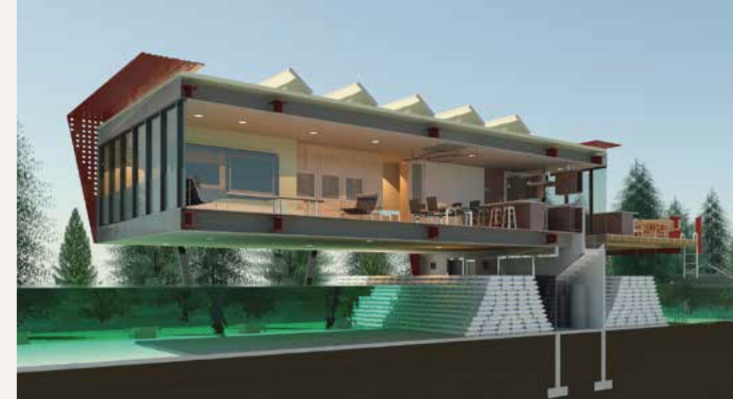
The "Flood House" was the first residential dwelling concept that F9 created to withstand a natural disaster. It rises above the ground while still offering all the comforts of a modern home. It's a ramped-up version of the home model people living in marshy areas have used for centuries, but with added protective and sustainable features, as well as style.
