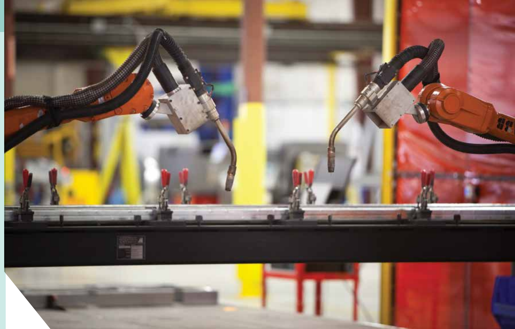
In lieu of the traditional craftsman welder, Prescient has utilized programmed robot arms to bring a new level of precision and accuracy to the welds on each piece of structure.
