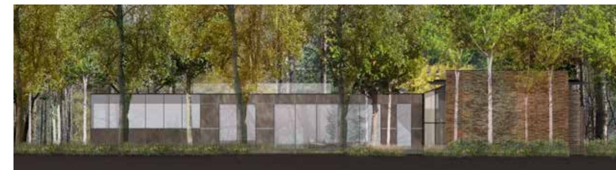
The renovation of the Lundy house by 1 Friday Design will closely resemble the above rendering. The north, or Lake Avenue elevation, highlights the continued use of lighting as vignette. The existing brick structure on the right will remain intact, along with the pitched-roof glass structure to its left. Stretching a whopping 70 new feet to the west, the addition’s height is kept at just 15 feet to honor the original design’s integrity, despite the approval to expand to 25 feet. And although square footage is tripled in the project—increasing from 3,508 to 9,000+ square feet—the reuse of composite materials ensures the essence of the original is felt throughout; bricks removed from an interior wall will be carefully preserved and reused in the renovation.
