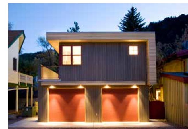
ABOVE TOP: The playful and exaggerated overhangs on this artist studio offer more than just a modern take on the traditional West End Victorians. Along with an interior slatted wall, the intentionally large gabled design creates naturally circulating airflow and assists in regulating direct solar gain. Also take notice of the recessed window; more than a unique detail, the design provides privacy from a nearby development. ABOVE BOTTOM: The Work N Park Cube is a playful garage and office solution for a shared condominium unit in the West End. The alley building integrates a LEED-inspired approach, including solar strategies and rain collection integration.
