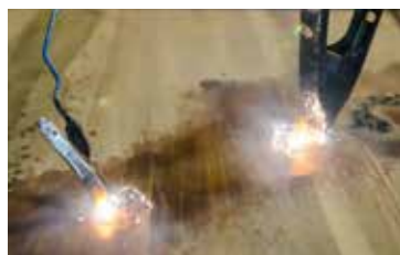
Designer James Davis had been experimenting with electrical erosion for about six months before meeting Vertical Arts' Brian Patty at a networking event. They quickly devised a plan to incorporate the technique into a multi-purpose table for VA's new office space. Using a solution of baking soda and saltwater to provide a general pattern, electrical clamps run through a series of microwave transformers to create a unique design on walnut butcher block.
