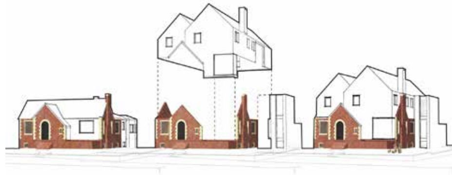
This schematic shows how the project unfolded. Architect Adam Harding of Roth Sheppard took the basic form of the original brick house, including the front facade, and added a gabled second story that includes three bedrooms and baths.
