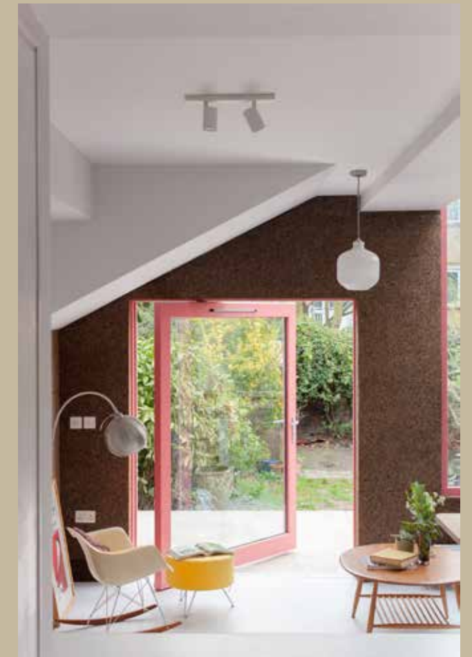
Naturally stained cork clads the interior and exterior walls of this extension to a Victorian terrace house in South London designed by Nimtim Architects. The exterior cork complements the home’s existing brickwork and will weather to a silvery-gray over time. Also, because cork is naturally water-resistant and thermally efficient, the building does not require extra foam insulation. Photos by Megan Taylor.
