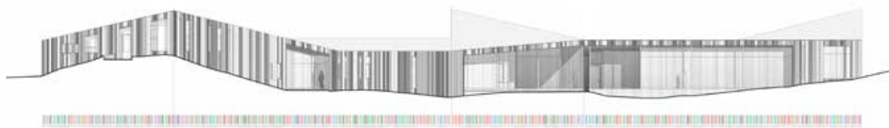
The siding profiles of the copper-clad exterior are arranged in the pattern of the DNA sequence of the Engelmann spruce, creating subtle modulations of light and shadow. Copper was selected for its resilience and ability to naturally patina over time. The steel roofline shifts and folds to follow the undulating topography of the site.
