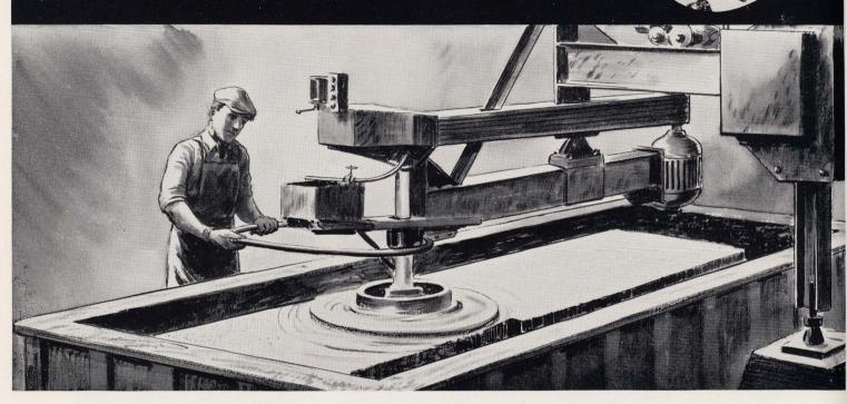
• Carbolon GP meets the challenge of granite polishing because each individual grain, approaching the diamond in hardness, is sharper and harder than the crystals of quartz that characterize enduring granite. specially processed and shaped to withstand the extreme pressure of the scroll wheel. They effect worthwhile economies, saving polishing time and abrasive materials, since less is required to surface a given area.
