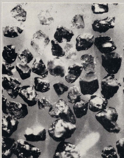
BLASTITE GRAIN, 30 grit, under the same magnification, shows its true abrasive qualities—sharp, angular fracture of every grain. Higher material cost is far outweighed by the much shorter labor time.
