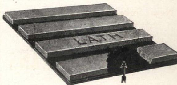
*Shows construction of Bishopric Sheathing. Arrows point to Asphalt Mastic into which laths are imbedded.*
