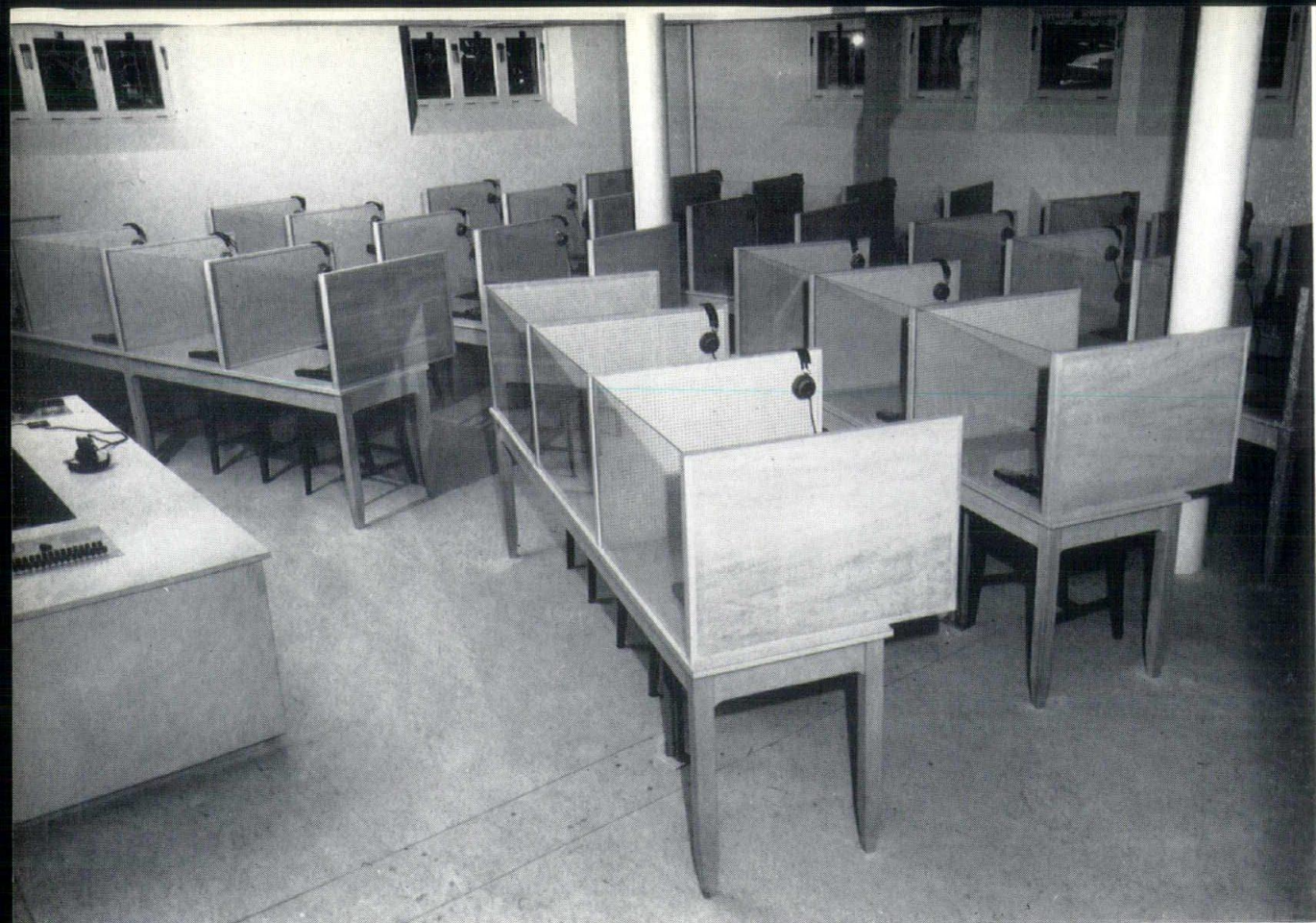
A Typical Language Laboratory Installation. The twenty-eight booths are of wooden construction with glass fronts to permit vision ahead, arranged in a chevron formation with aisles in the center and at either side. The central console, at left, contains master lesson distribution facilities (far side) and the intercommunication and monitoring panel (near side). Fluorescent lights are used, the ceiling has been acoustically treated, and booth wiring is run in floor ducts.
