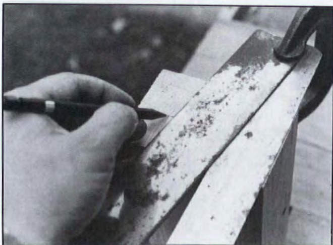
Below: The next step is to remove the copier and transfer the measurement to the new stock. (Be careful not to move the straight edges while working.)
