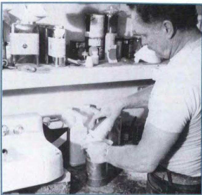
The two-part (resin and catalyst) polyurethane-based coating is mixed prior to spraying.
