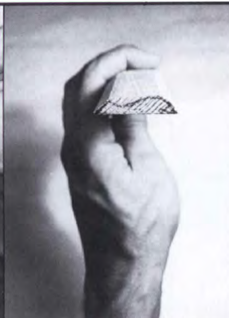
For a profile in square stock, plane straight and convex surfaces first.
