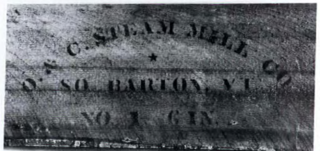
A mid-19th-century machine-made clapboard. The stamp "No. 1" or "No. 1 soft" always meant top-quality pine.
