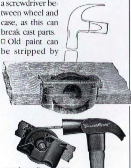
screwless pulleys c. 1898 mounted with special tool (top) and nail set (bottom)
