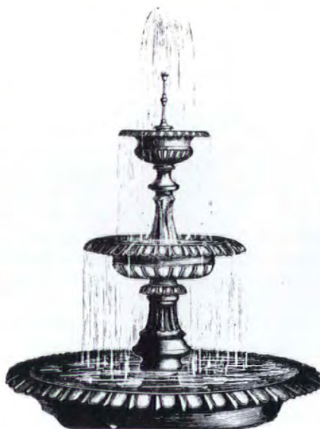
Fig. 7: A typical "3-spill" fountain, here 36 inches from fountain tip to the ground.
