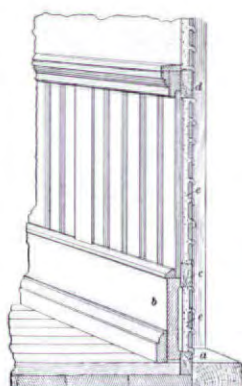
Grounds in plaster at d, c, & a anchor wainscot.
