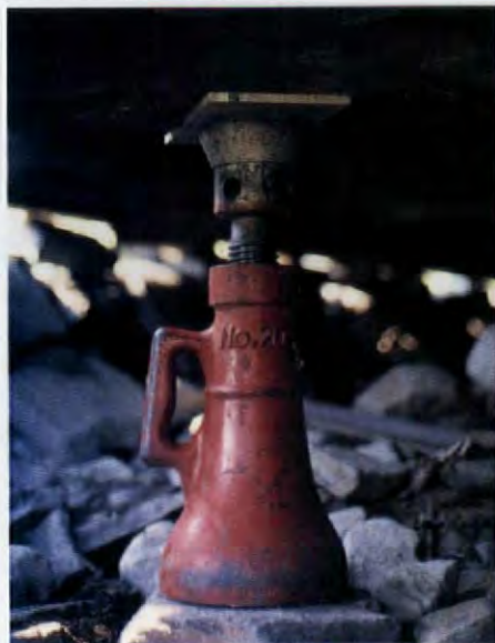
Left: When possible, use a bearing plate ( \frac{1}{8} "- \frac{1}{4} " steel plate) between the jack and the work to distribute the force of the jack over a broader surface. Right: Always stand clear of the bar or lever when jacking, in case it kicks back or gives way suddenly.
