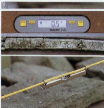
Top: An electronic level comes with a digital readout. Bottom: a line level attached to a mason's line.
