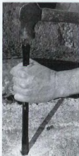
Star drills are hand tools that operate like chisels.
