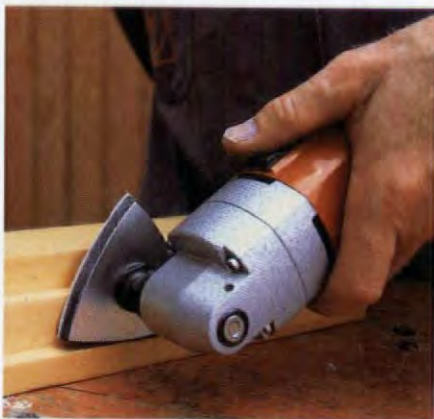
The three-pound Fein Sander can be used on wood, plastic, or metal surfaces.
