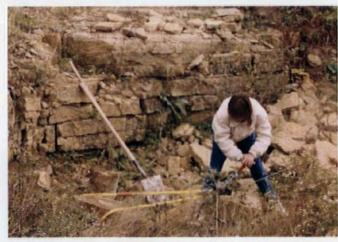
Exploit the natural breaks of horizontal bedding planes by wedging with chisels. A hand winch helps when loading stone.
