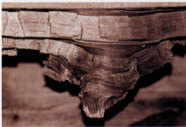
Fungal decay in wood typically produces a chunky, cubic texture. The lower half of this joist has crumbled away, leaving the resin-heavy knot.
