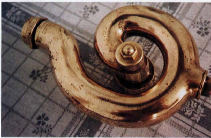
First patented in 1886, this P-style trap is still in working condition.
