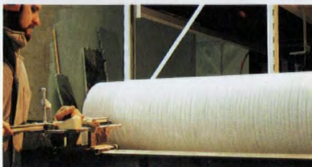
(top) Initially, the lathe is only used to mark the stone and establish round for the chisel work. (above) Later, the lathe is used continuously for final shaving of the workpiece to finish round.
