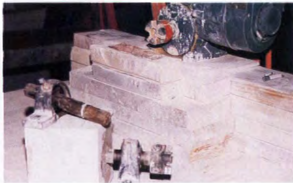
The motor/coupler assembly as well as the pillow blocks must be raised to the correct height (lumber works well) for the bit to cut properly.
