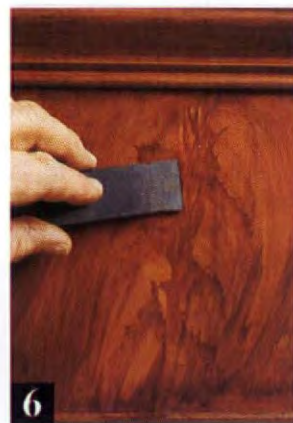
6 Using a piece of rubber, cardboard, or plastic wrap, wipe out the light highlights that radiate up and out from the center of the figuring.
