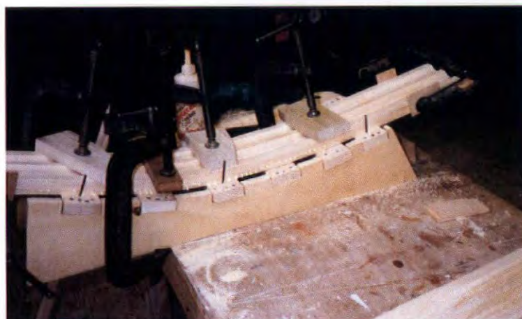
Laminating a moulding requires gluing several thin pieces together and thoroughly clamping them in a form, a method that produces stronger results than kerfing.
