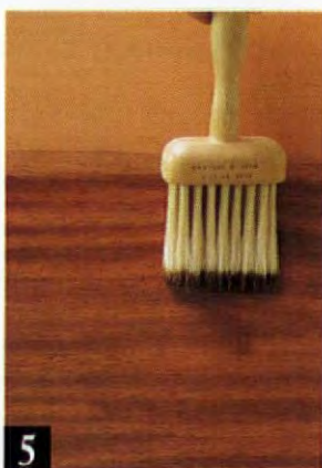
Just before the patterning sets up, soften the markings perpendicularly or opposite the grain.
