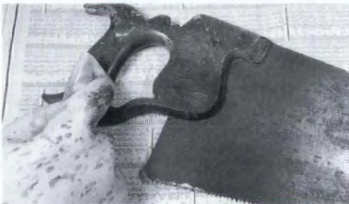
Clean up handles with turps or mineral spirits (above); finish bare wood with tung oil. Mild kinks (below) may flatten in a cushioned vice.
