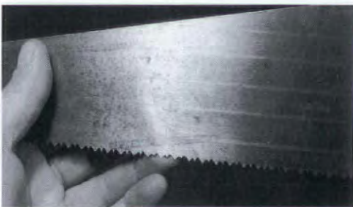
Clean up handles with turps or mineral spirits (above); finish bare wood with tung oil. Mild kinks (below) may flatten in a cushioned vice.
