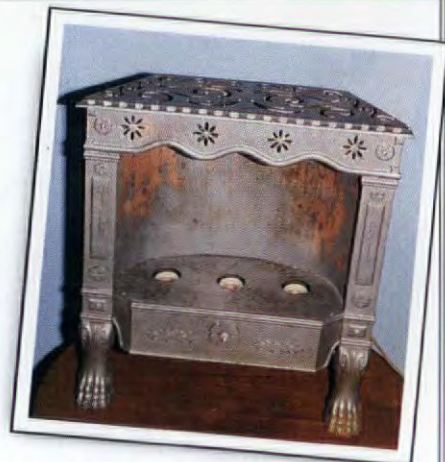
An early electric heater, missing its screw-in heating elements.
