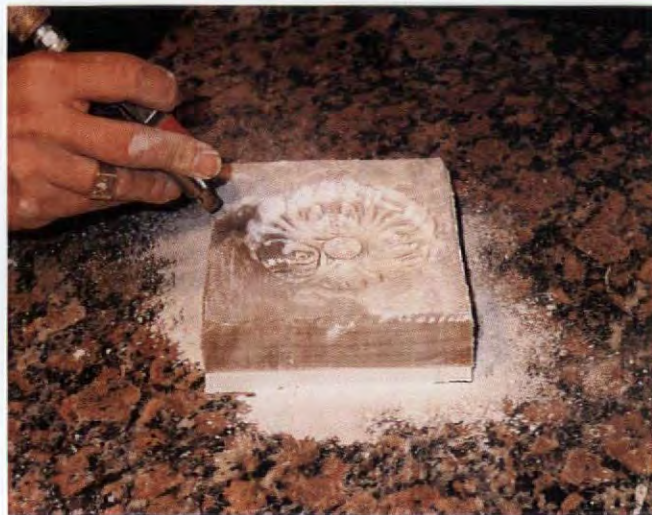
The separating solution has to be removed before the protective alum coating can be applied. Dust the surface with French chalk, then blow it clean.
