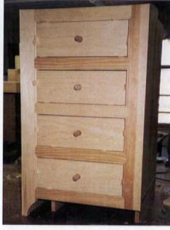
Attach drawer heads after cabinet is assembled. Use small spacers to ensure that they are centered. Note the turned wood pulls, a good "Shaker" cabinet detail.
